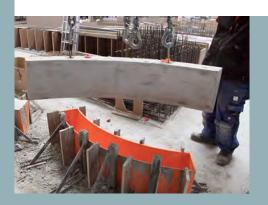
3D printed patterns and molds can replace expensive CNC milled or hand-crafted traditional forms. By modernizing the first phases of numerous casting applications, the BigRep ONE allows you to produce in-house, iterate faster, cut material costs, and streamline logistics. BigRep customers use the ONE to print forms for making carbon-fiber parts like drones and custom auto bodies, for various kinds of concrete casting, and to produce patterns fo anything from bathtubs to propellers.
